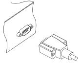
Plug one end of a RS-232 cable (9 pin D-sub cable) into the RS-232 port on the digital receiver, and the other end into the matching port on your computer.
